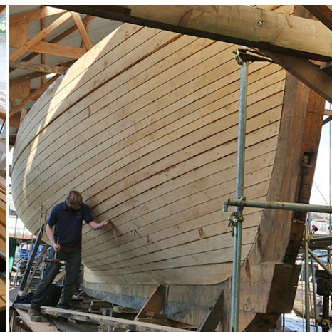
Photo 9: (L to R) Laying the opepe deck planks; planking complete and caulking under way.
