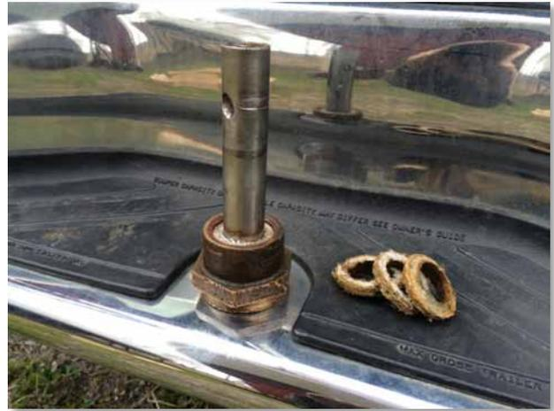
Installing the new cutlass bearing was the reverse of removing the old. The new bearing was first positioned in the stern tube, then the collar was replaced and the Allen screws were tightened down to hold everything in place. Care must be taken to tighten the Allen screws enough to be snug and not vibrate out, but not so much that they deform the cutlass bearing.
