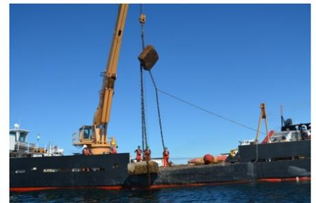
*Buoy deck personnel aboard the Coast Guard cutter Mobile Bay, a 140-foot icebreaking tug, retrieve two 5000 pound sinkers Aug. 26, 2015, at Fisherman Shoal Lighted Bell buoy 6 in Lake Michigan.*
