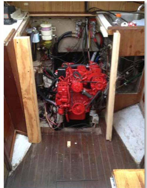
*Cabinetry modifications to accommodate the new motor, which is slightly larger and has accessories in different locations.*
