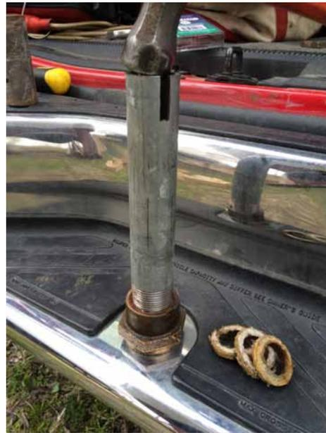
The hole in the rear bumper of my van happened to be the correct diameter to support the shaft and hold the packing nut in place while the stuffing was pressed into place. If you notice, the pipe I was using is slotted for use as a tool to install or remove 1½-inch thru-hull fittings.
