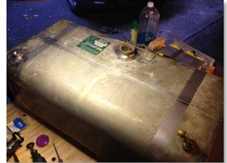
After cleaning out the tank and letting it dry, some sediment could be heard rattling around in the tank when it was rocked back and forth. Because the fill tube extended nearly to the bottom of the tank, it was decided to cut an access/clean-out port into the top of the tank. This was done with a Dremel® Tool and an abrasive cut-off wheel.
