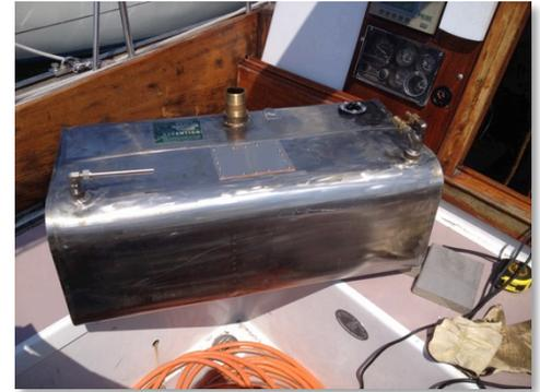
Reinstalling the tank in the boat went a lot easier than removing it. This was partly due to the fact that we were not reinventing the process but simply reversing it. The tank slid back into the port cockpit locker easily and then into its cradle from there. All fittings had to be removed for this maneuver, but once the tank was in its cradle, they were easily reinstalled and tightened down.
