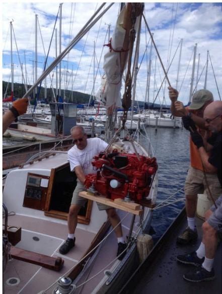
While four people could lift the engine on its pallet on dry land, doing so to transfer it to a boat floating in a slip was not practical, so step one was to place the motor on the dock where it could be picked up from the boat. The slip used by our marina travel lift was chosen
