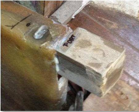
With the engine bed marked, reinforcing "backers" were then epoxied into place. Given the geometry of the hull, it would be impossible to use regular machine bolts to secure the engine
