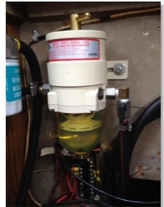
To meet these needs, we elected to mount the fuel filter/separator (a Racor 500) next to the oil filter in the engine space. A small shut-off valve can be seen on the inlet to the filter so that the canister will not overflow when filters are being changed. (The filter is actually at the same level as the fuel tank, so if the tank is full, the canister will overflow if the top is opened for filter removal.)
