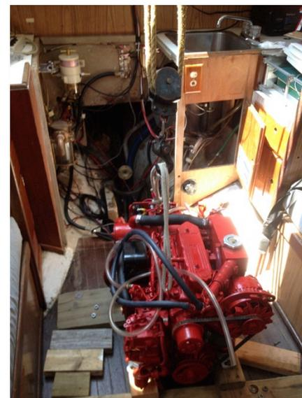
coupling in the drive train increased this difference by a little over 3 inches. Also worth noting (as it becomes significant in the next paragraph), is that the alternator is located on the port side of the motor, opposite that of the Atomic Four.
